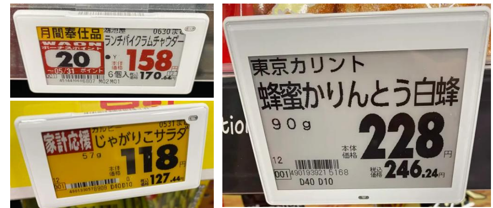
Wireless electronic shelf labels at AEON in Nagoya
